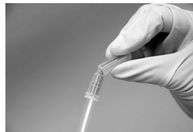
Snap the liquid-filled bulb
